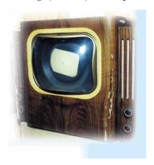
In 1954 Russia built its first color sets. Named "Raduga", which means rainbow, the sets used the field sequential method. This information is from various Russian websites, one of which has a <u>description</u> (in Russian) of the system. The system was experimental, and only a few sets were made. Here are a <u>technical manual</u> and a <u>page describing the set</u> (in Czech). Here are photos of a surviving set at the <u>Popov Museum</u> in St. Petersburg, Russia.
